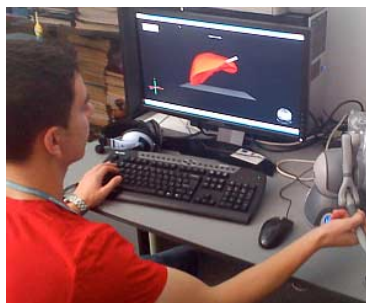
Figure 3. Student experimenting with the haptic liver palpation simulator.
